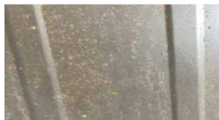
Heavy swarf staining on pre-painted ZINCALUME.
