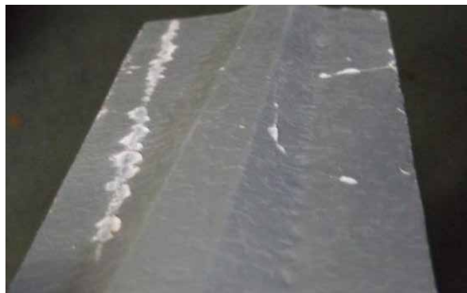
Note that when scratched, the primer has been compromised as well as the presence of Zinc Oxide (white rust).
