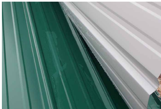
This method traps moisture underneath. After just 3 months covered in the manner above, the panel bundle is opened to reveal that moisture has made its way into the layers of sheets.
