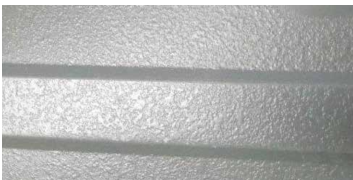
Close up image of severe "Wet Stack Corrosion". Note smooth, normal surface in upper right corner.
