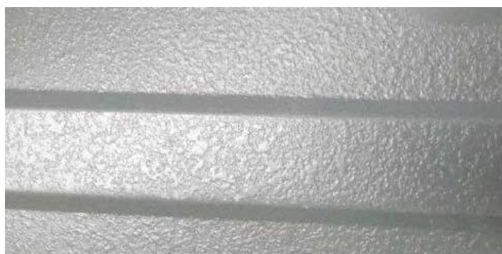
Close up image of severe "Wet Stack Corrosion". Note smooth, normal surface in upper right corner.
